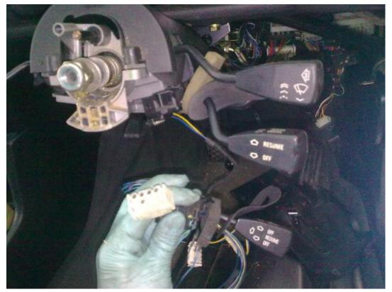
\* The earlier cruise switches have less wires in a different arrangment to the later cars (5 wires in a T formation)
