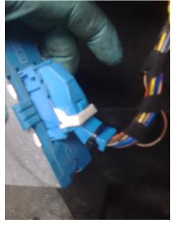
• Pop the ECU into the inner body, screw plastic nut back on to secure the holder . Yellow wire coming towards the camera is for the speaker
