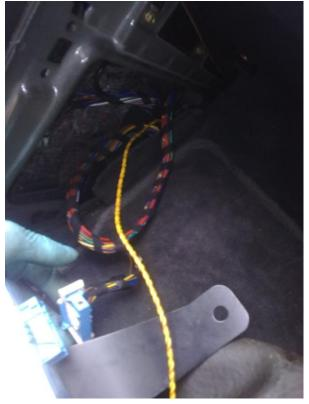
• With cruise ECU in holder connect to loom with the appropriate numbers meeting (1 to 13 one side 14 to 26 the other IIRC)
