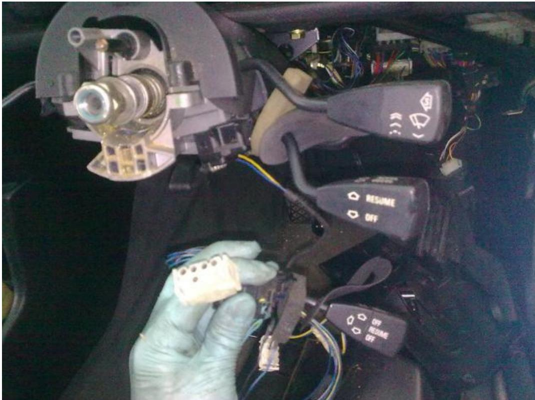
\* The earlier cruise switches have less wires in a different arrangement to the later cars (5 wires in a T formation)
