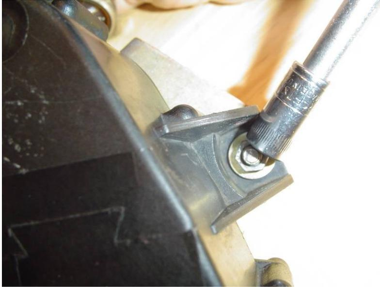
**Figure 13 - Remove mounting plate nuts**
