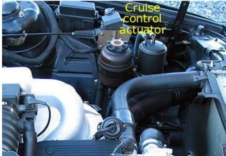
**Figure 25 – Typical E34 mounting (non-540i)**
