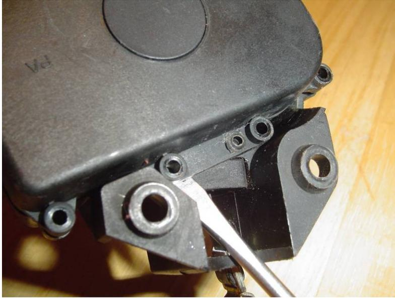
**Figure 15 - Using screwdriver to separate shell halves**
