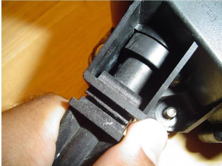
**Figure 10 - Sliding out throttle cable**
